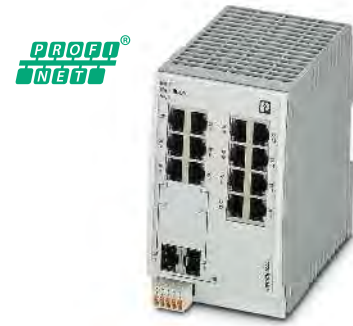
14 RJ45 ports and 2 SFP ports 10/100 Mbps
