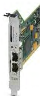
Router with firewall and VPN for PCIe
