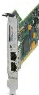
Router with firewall and VPN for PCI
