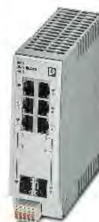
6 RJ45 ports and 2 SFP ports 10/100/1000 Mbps
